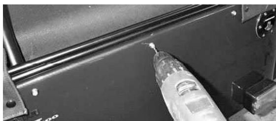
Fig 22 Drilling central popper on SV
