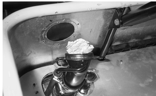
Fig 15 Old filler boss removed
