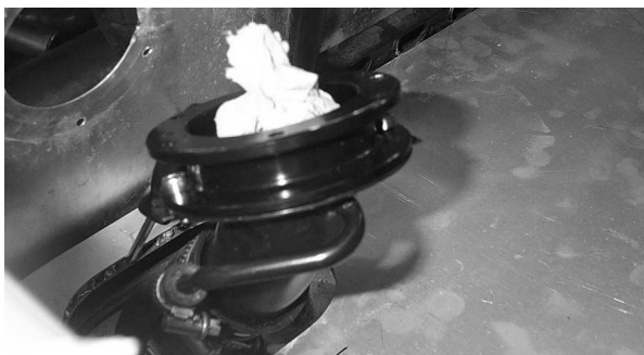
Fig 18 Spacer fitted to filler neck
