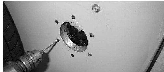
Fig 14 Drill out the six rivets
