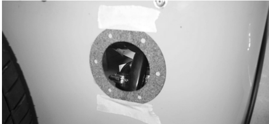
Fig 16 Gasket positioned on back panel
