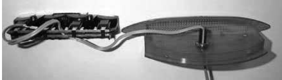
Fig 24 Wire routing through light unit
