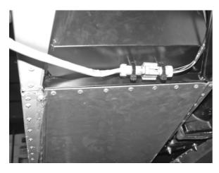
Fig 11 Lambda probe connection
