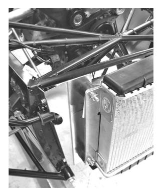
Fig 17 SV radiator arrangement
