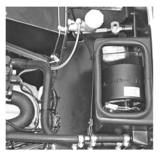
Fig 8 Clutch hydraulic hose
