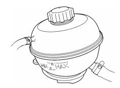
Figure 15: Coolant, Expansion bottle
