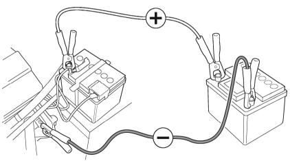
Using jump leads from a donor battery, or a battery fitted to a donor vehicle, is the only approved method of starting a car with a flat battery. Push or tow starting is NOT recommended!
