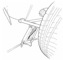
Figure 20: Rear jacking point
