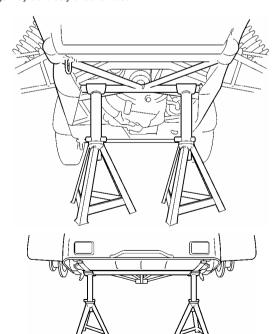
Figure 12: Rear Axle Stand Positioning
