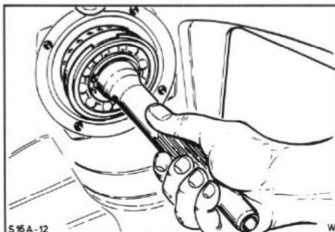
Fig. 138. Slide input shaft into housing.
