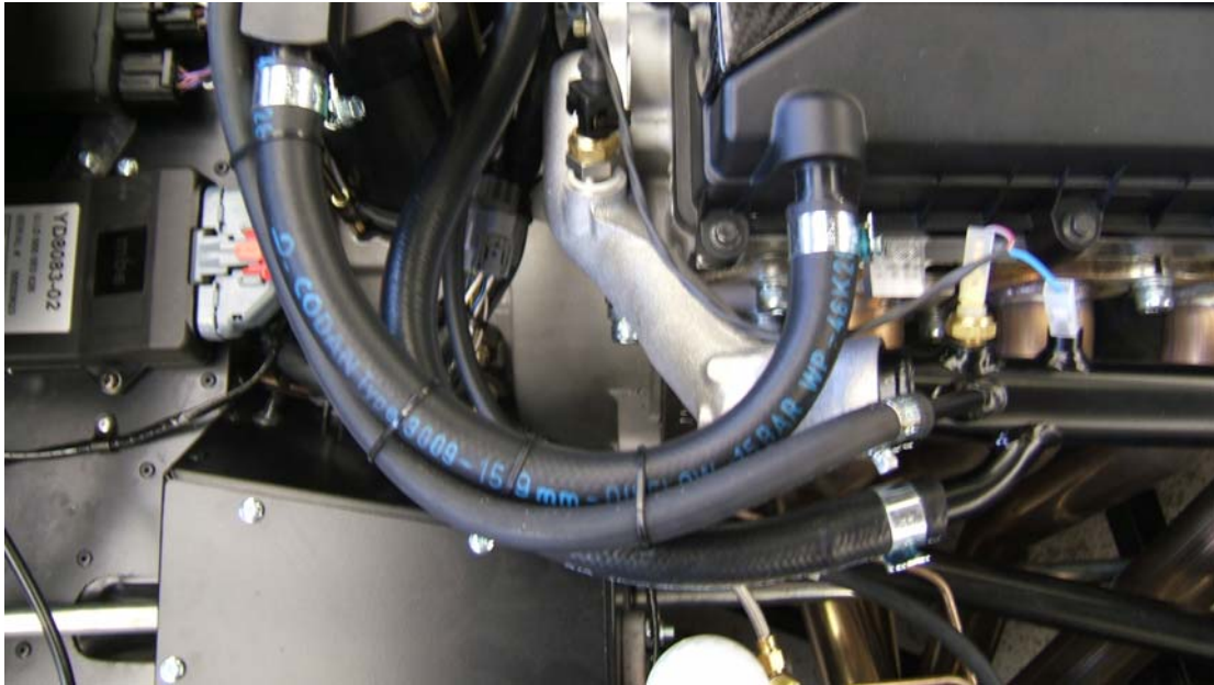
Figure 22 - Cam cover to swirl tower breather system
