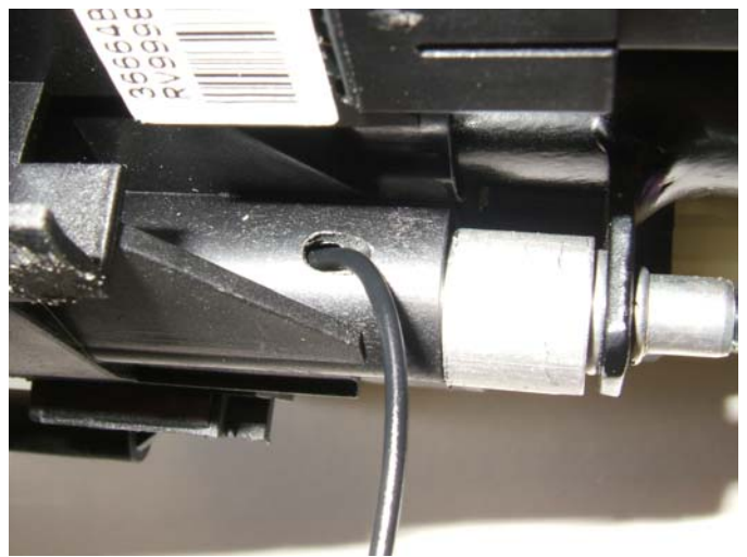
Figure 42 – Wire position for contact pin
