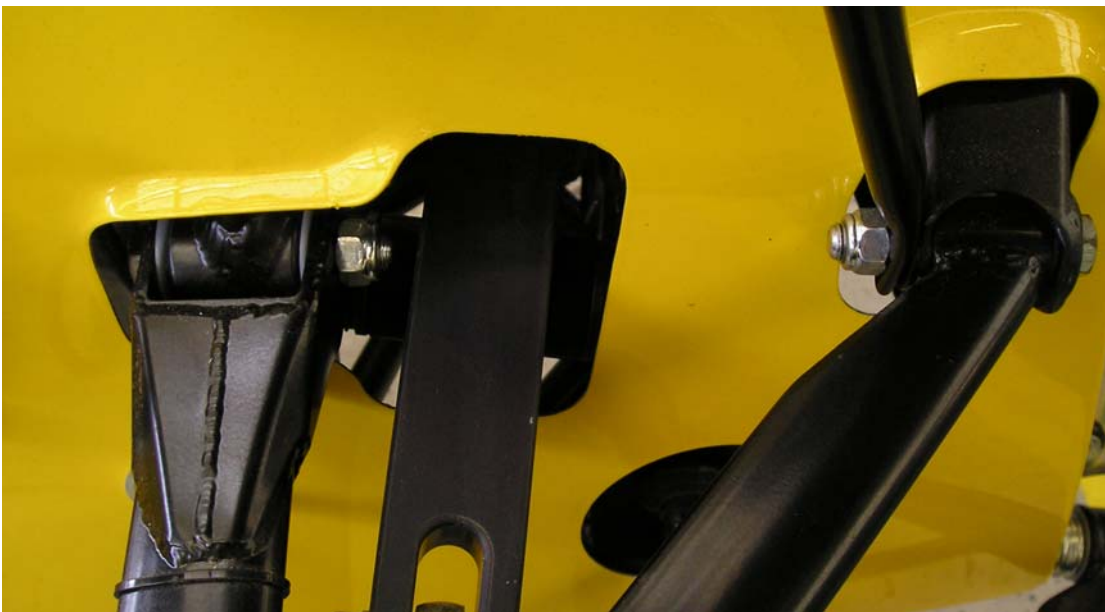
Figure 1 – Top wishbone assembly detail
