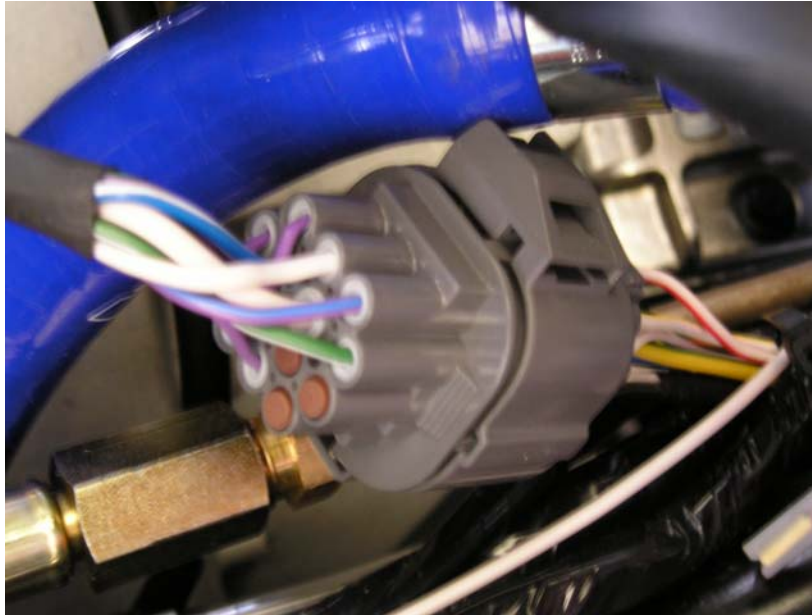
Figure 33 – Grey multi pin plug to connect the vehicle and engine harness together
