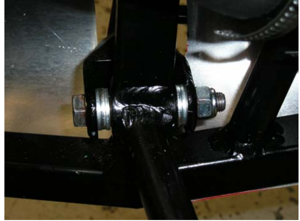
Figure 3 – Front lower wishbone assembly (rear joint)
