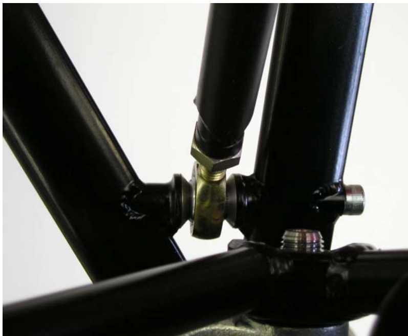
Figure 6 – Push rod to lower front wishbone joint
