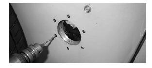
Fig 14 Drill out the six rivets
