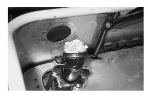
Fig 15 Old filler boss removed
