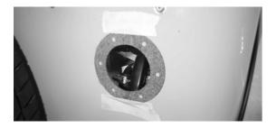
Fig 16 Gasket positioned on back panel
