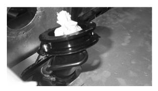
Fig 18 Spacer fitted to filler neck
