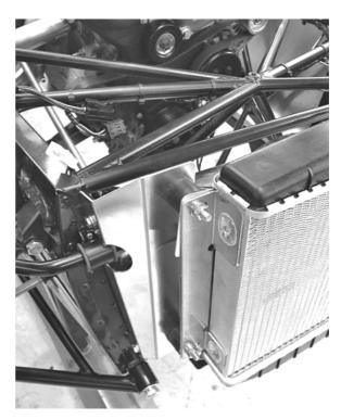
Fig 17 SV radiator arrangement
