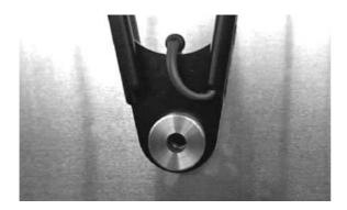
Fig 28 Wires from support tube entering boot
