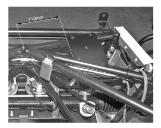
Fig 2 Header tank location plate
