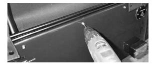
Fig 22 Drilling central popper on SV
