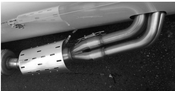
Figure 44: Primary pipes and collector/catalyst
