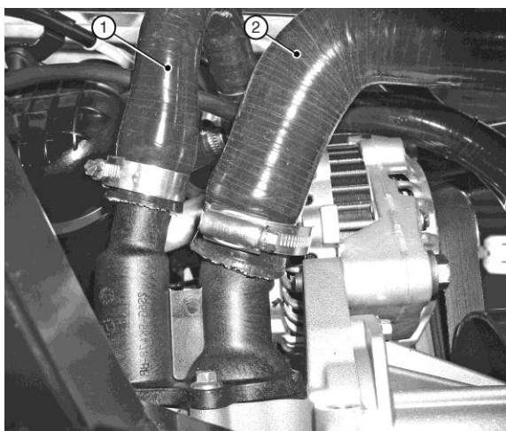
Figure 48: Bottom hose engine connection (viewed from bellow)
