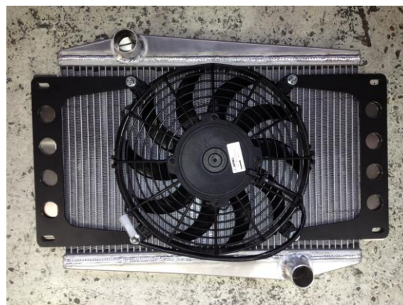
Figure 49: Radiator/fan prior to fitting
