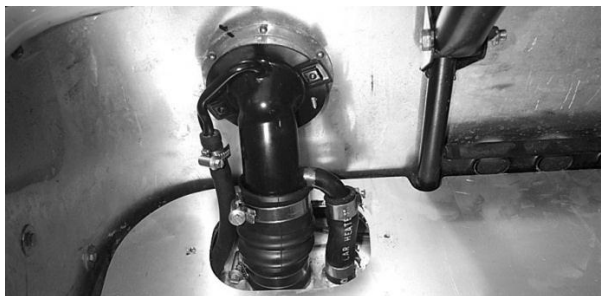
Figure 182: Filler cover and boot carpet removed
