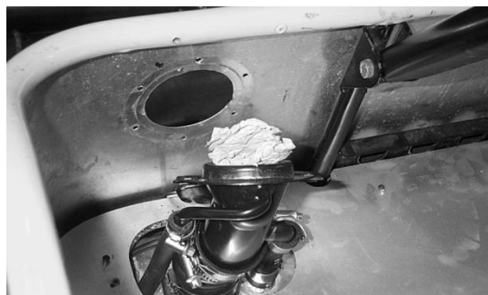
Figure 184: Old filler boss removed
