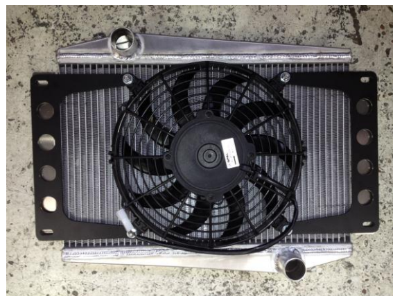
Figure 49: Radiator/fan prior to fitting
