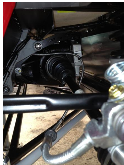
Figure 132: Handbrake cable routing S3 (non-adjustable side)
