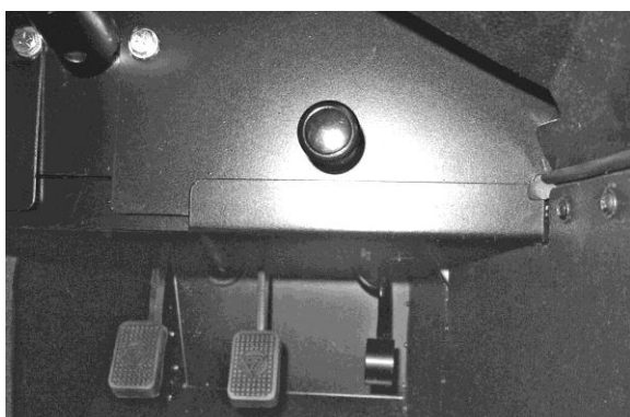
Figure 82: Heater control location
