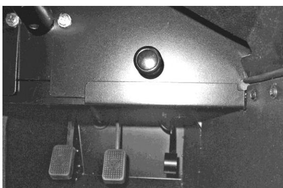
Figure 55: Heater control location
