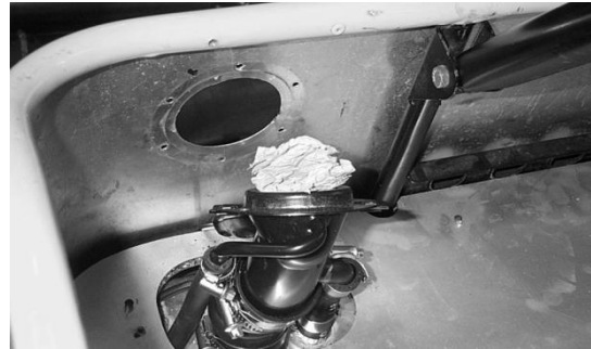
Figure 184: Old filler boss removed
