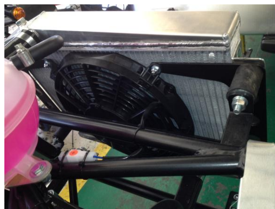
Figure 50: Standard radiator arrangement
