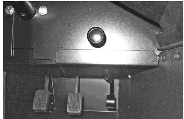
Figure 115: Heater control location
