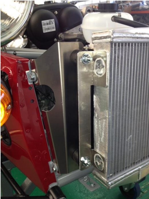
Figure 56: SV radiator arrangement
