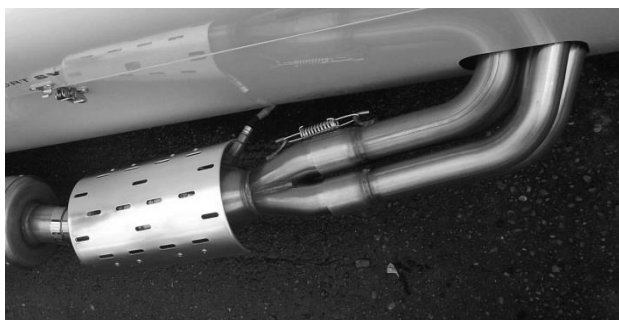
Figure 49: Primary pipes and collector/catalyst
