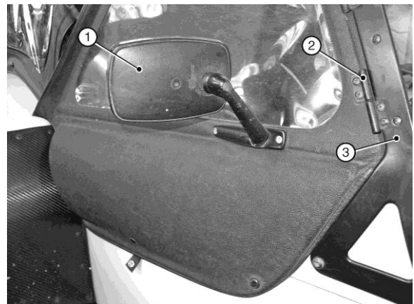
Figure 166: Mirror fitted to side screen
