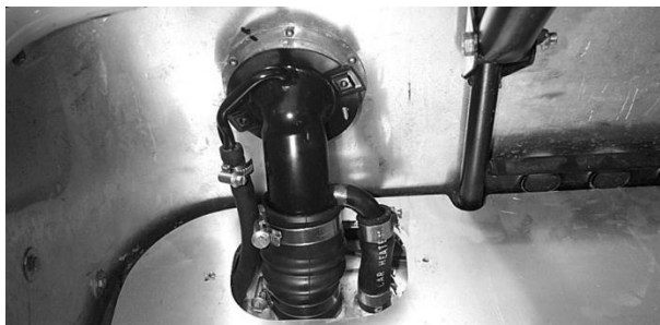
Figure 188: Filler cover and boot carpet removed
