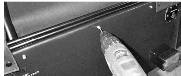
Figure 197: Drilling central popper on SV
