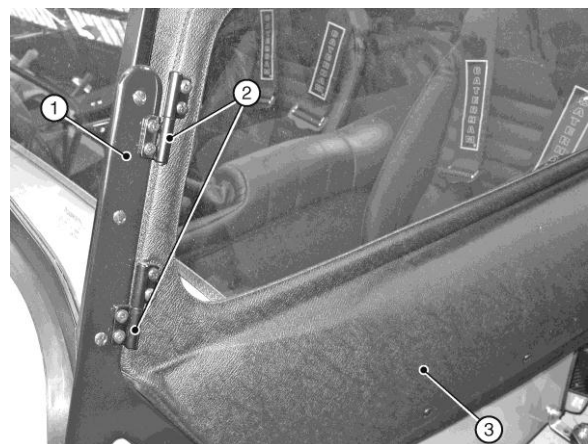
Figure 162: Hinge and side screen fitting
