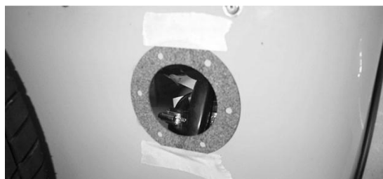
Figure 191: Gasket positioned on back panel
