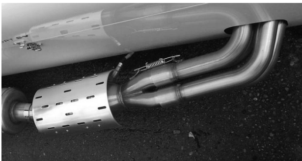
Figure 49: Primary pipes and collector/catalyst
