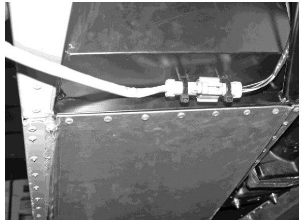
Figure 50: Lambda probe connection
