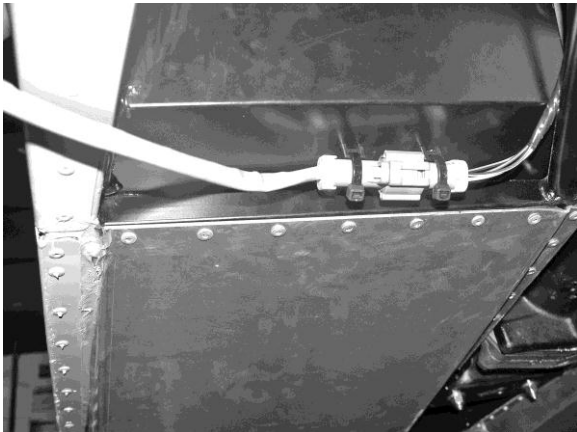
Figure 77: Lambda probe connection
