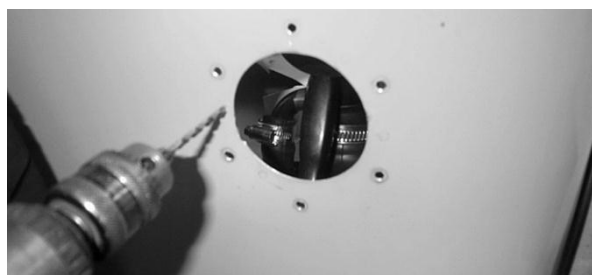
Figure 192: Carefully drill new holes
