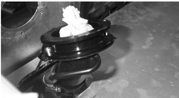
Figure 193: Spacer fitted to filler neck
