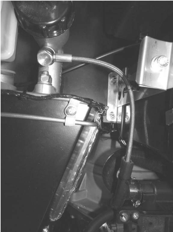
Figure 101: Clutch hydraulic hose
