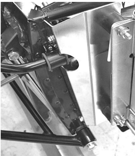
Figure 82: SV radiator arrangement
