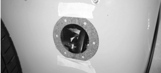
Fig 16 Gasket positioned on back panel
