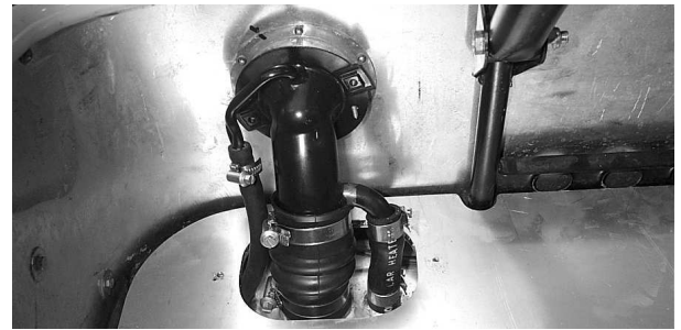
Fig 13 Filler cover and boot carpet removed
